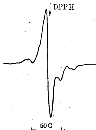
图2 芥子酸 77 K 辐照升至室温退火后的 ESR 波谱 Fig. 2 ESR Spectrum from Sinapic Acid irradiated at 77 K, recorded after annealing at room temperature
